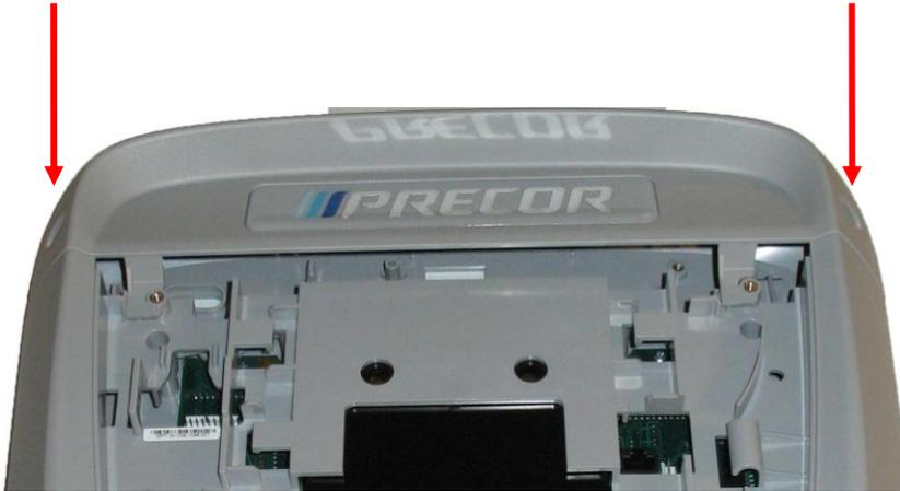
9. Remove the 6 screws that fasten the rear cover from the console and remove. **See Diagram 6.5.7.**
