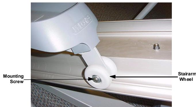
7. Slide the replacement wheel onto the stairarm axle. Fasten the wheel with the hardware removed in step 6. Apply blue loctite to the wheel mounting screws and torque them to 180 inch pounds.
