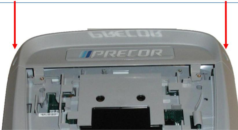
10. Remove the 6 screws that fasten the rear cover from the console and remove. **See Diagram 6.6.7.**
