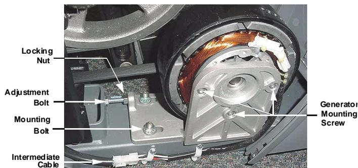
9. Set the replacement generator at its mounting position. Remove the three generator mounting screws, the two bearing clamp screws and the bearing clamp. Lift the generator and place the drive belt around the generator's pulley.
