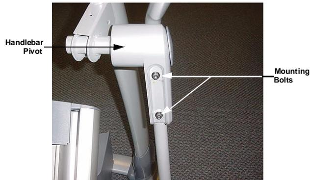
4. Set the handlebar at its mounting position and hand start the mounting bolts removed in step 3 that fasten the handlebar to the handlebar pivot. Do not tighten them at this time.
